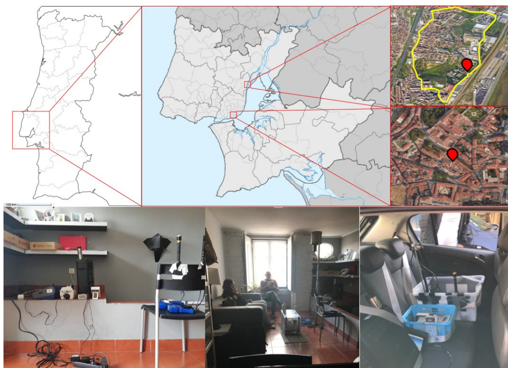
Figure 1. Top: measurement locations within the Lisbon metropolitan area (Portugal)—car route in Loures municipality ( right, top ) and location of the studied flat in Lisbon municipality ( right, middle ). Bottom: arrangement of the measuring instruments in the home ( left and center ) and car ( right ).
